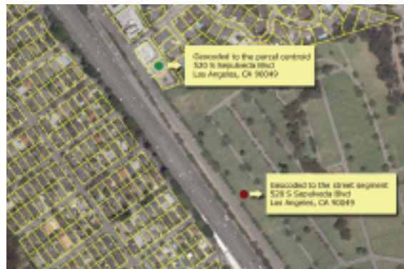
Even the best available street segment data can yield inaccurate geocoding results, in this case, over 900 feet.
